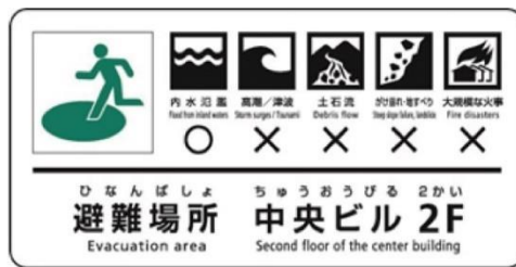
FIG. 2-3-3 Example of Information Board Using the Hazard Specific Evacuation Guidance Sign System
